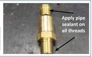
Re-tighten the orifice holder ensuring there is a small amount of pipe sealant on the threads.
