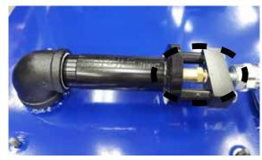
Inspect orifice for any debris. Remove the debris. If the orifice is severely plugged you may need to use compressed air. Check distance to inspirator.
