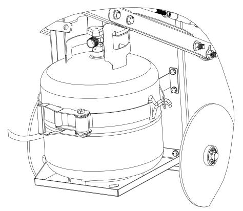
${\rm I}$  Only tighten the ratchet strap so that it is snug, do not apply excess force on the brackets
