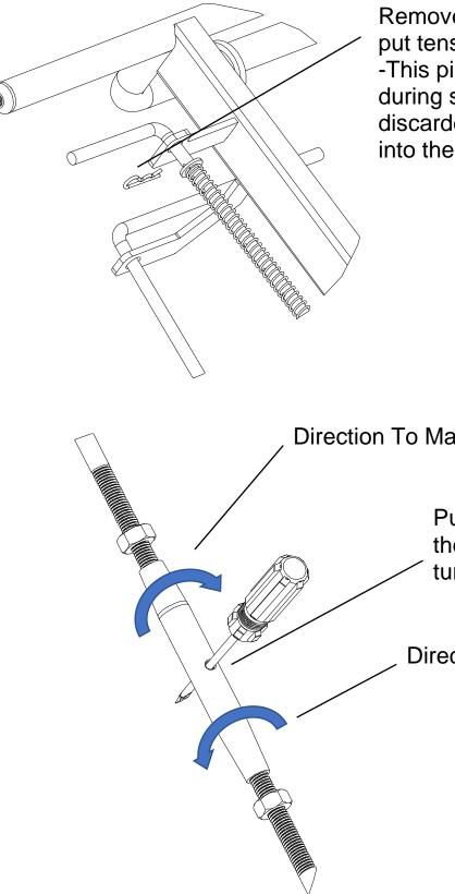
Remove the spring retainer pin to put tension on the valve control rod -This pin is just to hold the spring during shipping and can be discarded after installing the arm into the machine
