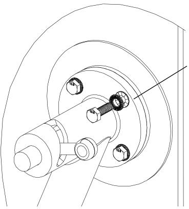
▲ The lock washers provided for the valve are shipped in pairs. Use 1 pair for each bolt with the wedged surfaces on the washers mated together (same orientation that the washers come paired in).
