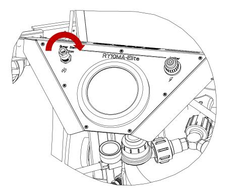
Simply thread the cap with your fingers over the button on the flame-out valve until snug. \*\*\*NEVER LEAVE THE EQUIPMENT UNATTENDED WHILE INSTALLED\*\*\*
