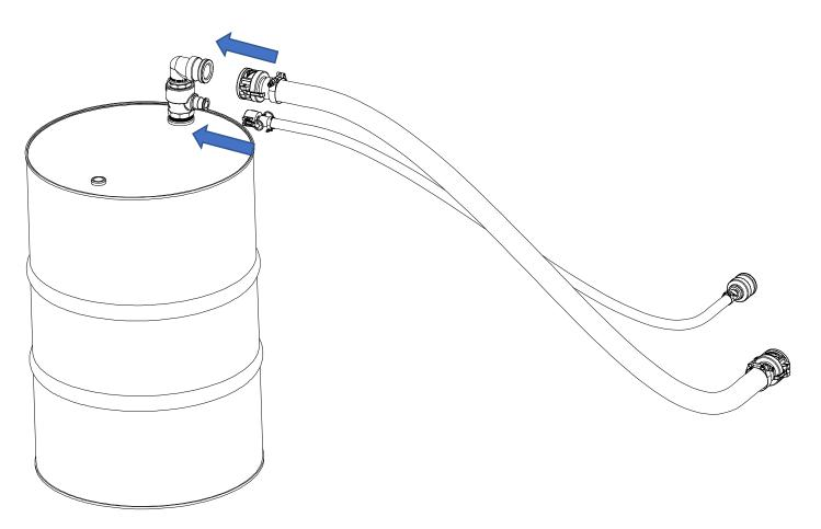
3. Connect the 2" male camlock connection to the pump valve and the 2" female camlock connection to the pump intake.
