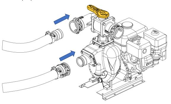
4. Connect the 2" male camlock connection from the spray wand assembly to the other side of the pump valve
