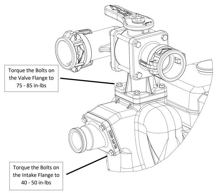
Use these torque specs with **ALL CAST IRON** systems (RA-SSY-0003, RA-SSY-0004, RA-SSY-0012, RA-SSY-0013, RK-SSY-0016, & RK-SSY-0017)
