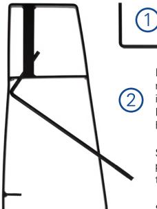
Screw the connector to the bottom of the "L" plunger handle.
