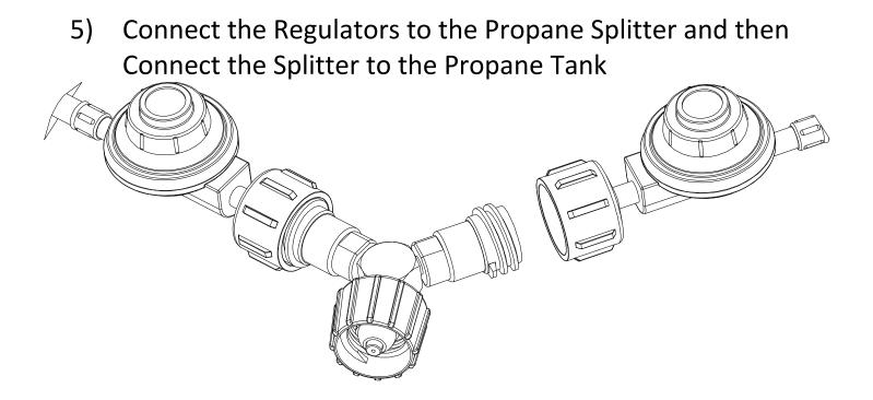
$\triangle$  Make sure to secure the propane hoses so that they are clear of the hot kettle walls during operation.
