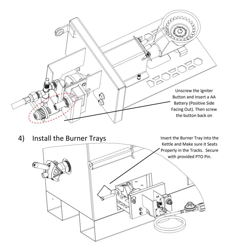
⚠ Make sure the burner trays are secured with the PTO pin at all times, especially during transportation and operation.
