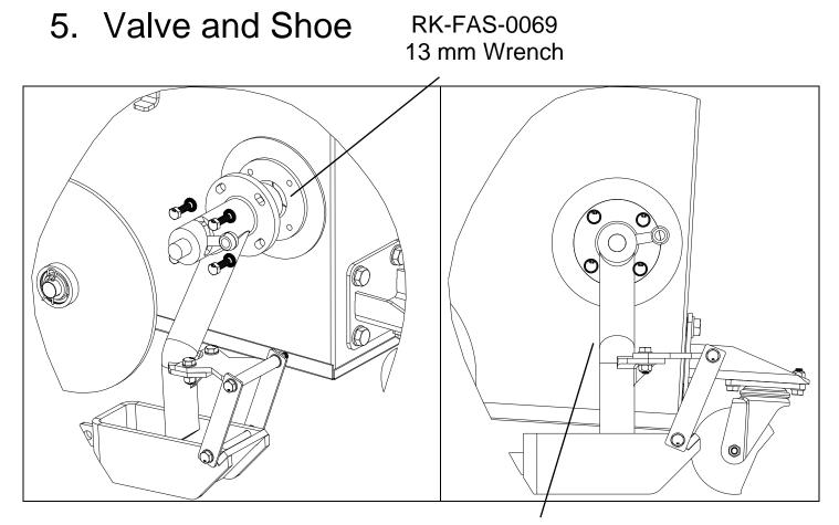
Valve should be aligned so it is perpendicular to the ground before the bolts are tightened
