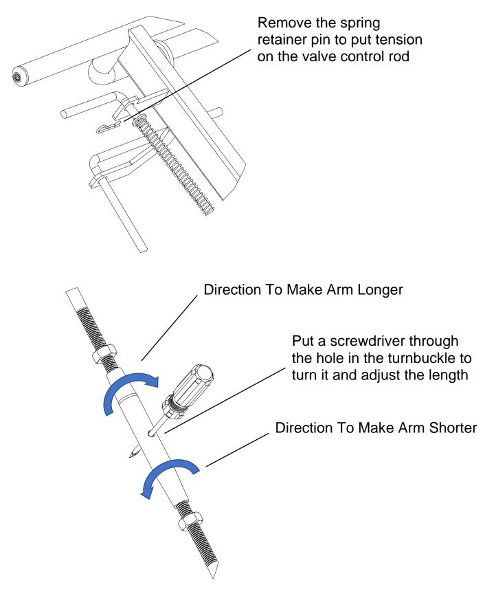
Adjust the length of the valve and shoe control rods so they are approximately in the position shown below.
