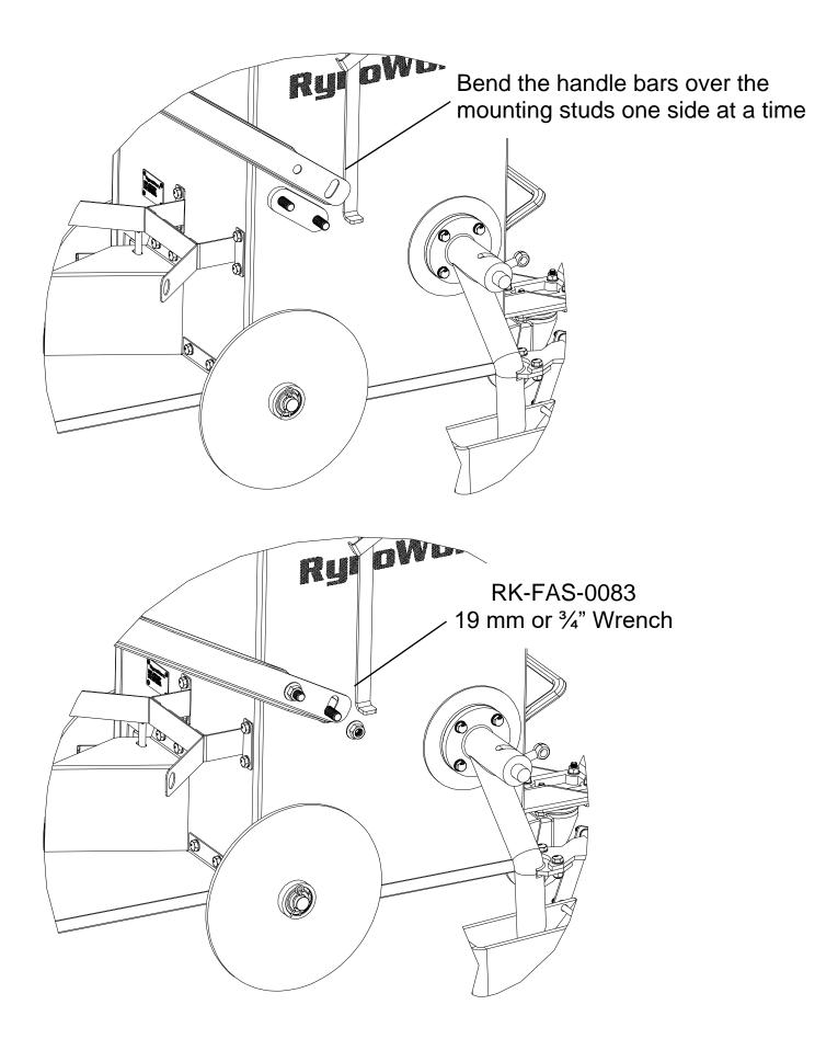
Tighten the handle bar nuts so that they are snug, nuts will be fully tightened in the set-up section.
