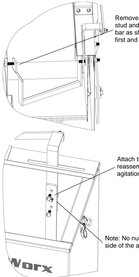
Remove the nut threaded on the stud and install the agitation sweep bar as shown, put it over the left stud first and then the right
