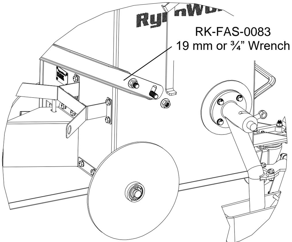
Tighten the handle bar nuts so that they are snug, nuts will be fully tightened in the set-up section.
