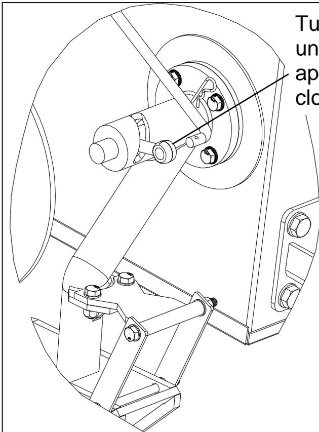
Turn the valve connector rod clockwise until it is tight and then turn it approximately 1 rotation counter-clockwise until its in the position shown
