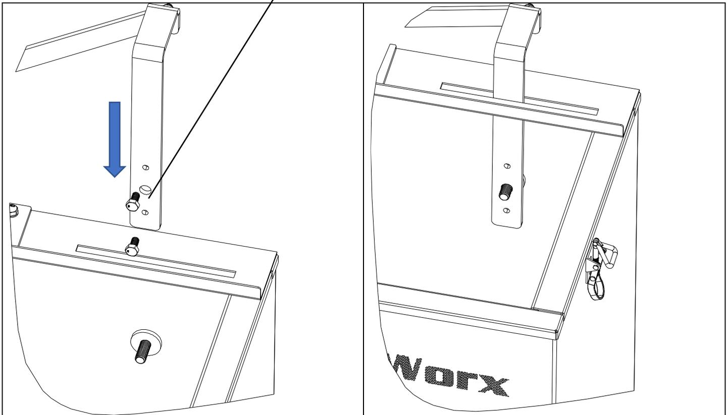
Remove the nut threaded on the stud and install the agitation sweep bar as shown, put it over the left stud first and then the right
