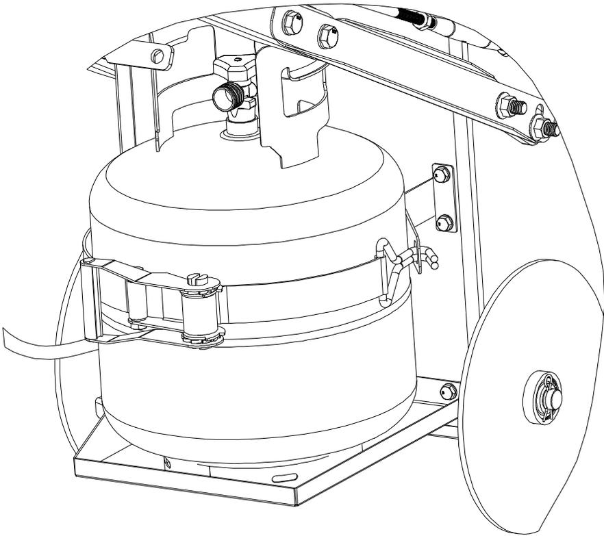
⚠ Only tighten the ratchet strap so that it is snug, do not apply excess force on the brackets
