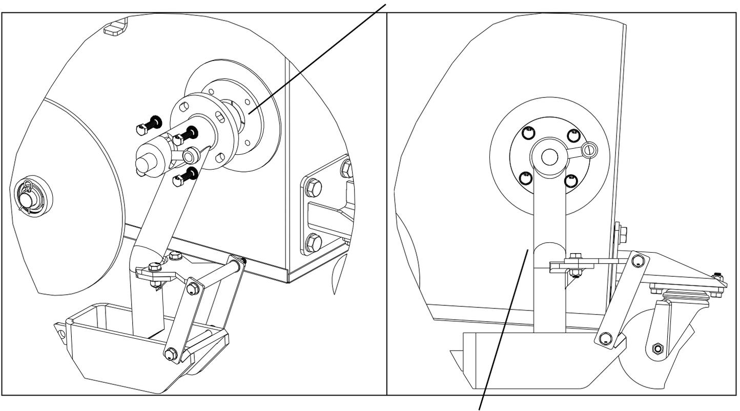
Valve should be aligned so it is perpendicular to the ground before the bolts are tightened
