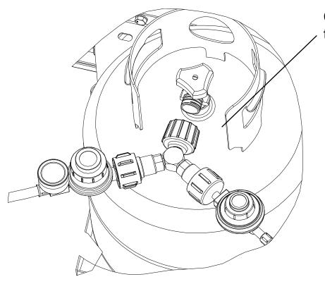
Connect the splitter to the propane tank
