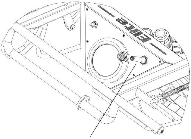
Unthread the igniter cap and insert the AA battery with the positive terminal facing up
