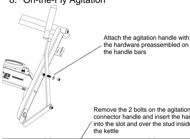
Remove the 2 bolts on the agitation connector handle and insert the handle into the slot and over the stud inside
