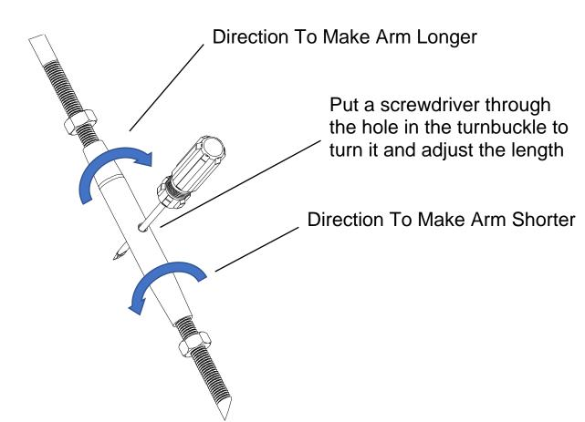
Adjust the length of the valve and shoe control rods so they are approximately in the position shown below.
