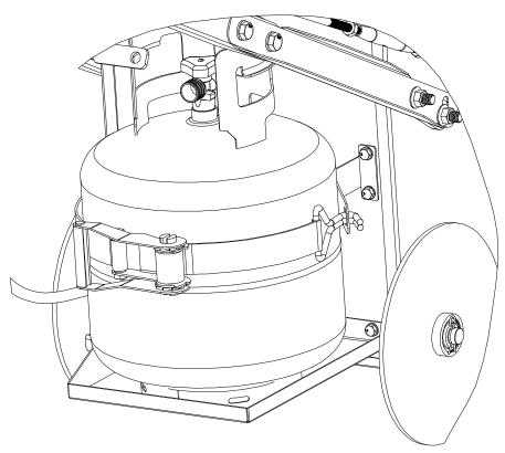
$\triangle$  Only tighten the ratchet strap so that it is snug, do not apply excess force on the brackets
