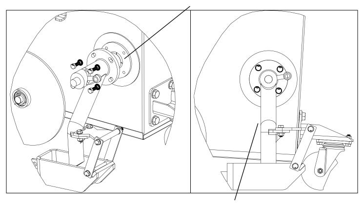
Valve should be aligned so it is perpendicular to the ground before the bolts are tightened
