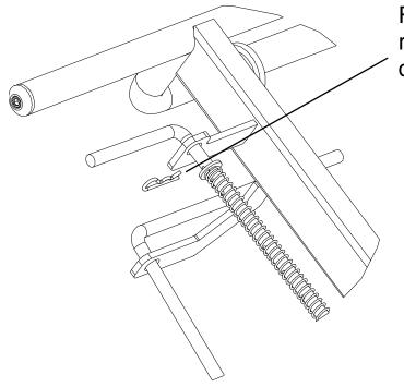
Remove the spring retainer pin to put tension on the valve control rod
