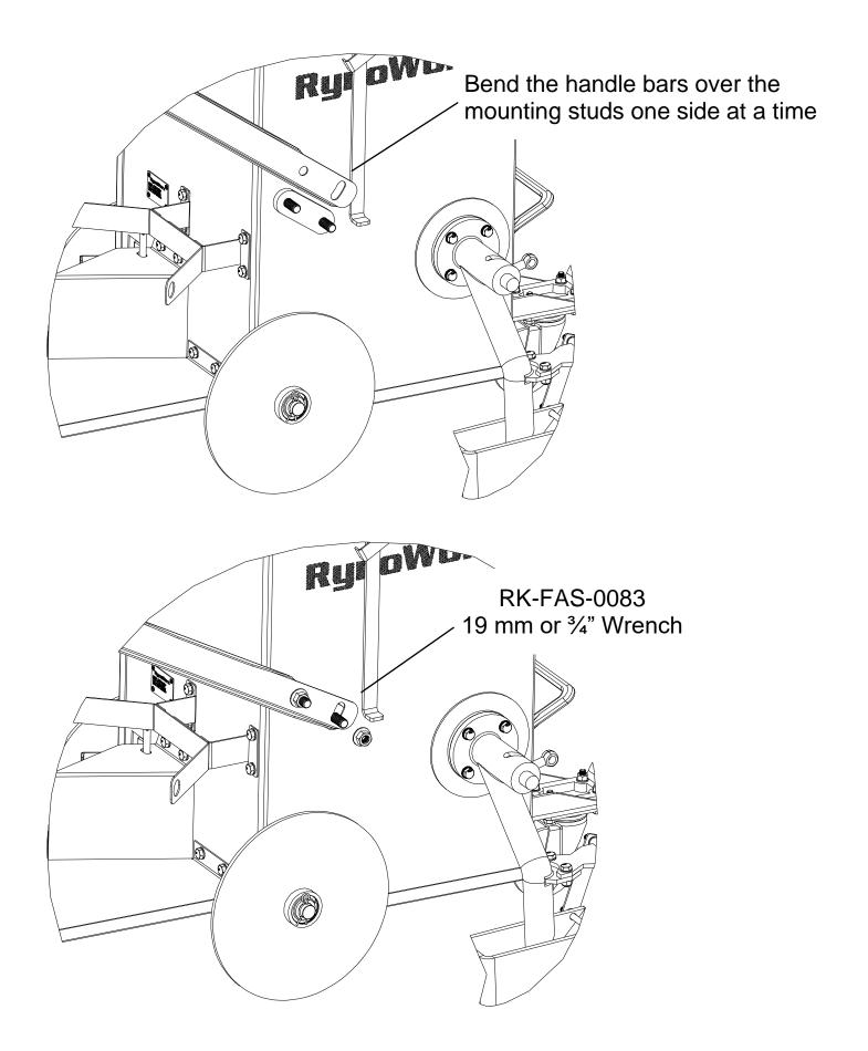
Tighten the handle bar nuts so that they are snug, nuts will be fully tightened in the set-up section.
