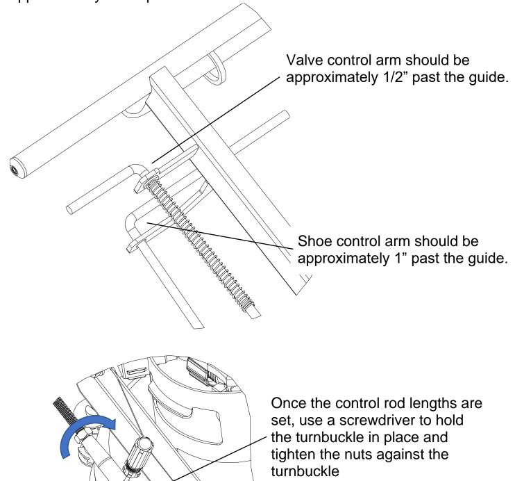
Set Up — Adjust Spring Tension
