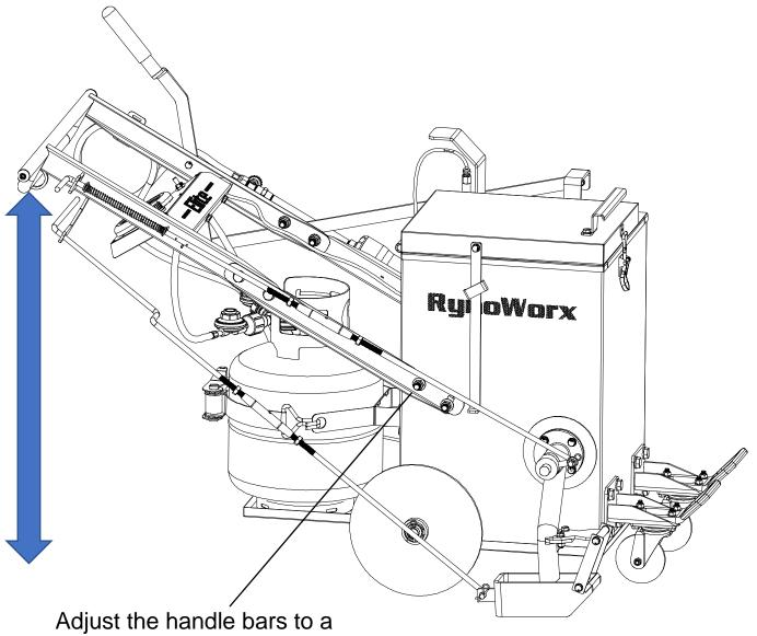
Adjust the handle bars to a comfortable height for the operator and tighten the flanged nuts on the studs (x2 each side)
