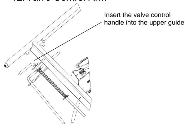
Turn the valve connector rod clockwise until it is tight and then turn it approximately 1 rotation counterclockwise until its in the position shown
